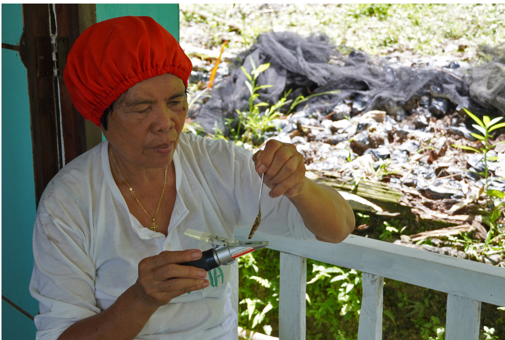
Macatumbalen village leader Nida Collado sits at the government-funded honey processing house as she measures honey moisture content with a refractometer to ensure it meets market quality standards. Photo by Keith Anthony S. Fabro for Mongabay.
