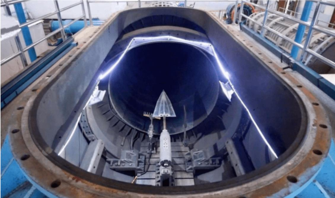
The older J-12 hypersonic wind tunnel in Beijing is working with the new facility to develop hypersonic aircraft. The JF-22 tunnel is capable of simulating flights at Mach 30 or 23,000 mph – 30 times the speed of sound. Credit: Handout
